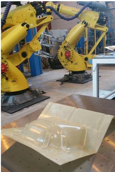
With the Elium® technology, Arkema offers a range of liquid thermoplastic resins processed by the same methods (resin transfer molding, infusion, flex-molding) as those used for thermoset resins, hence keeping down capital expenditure for processors.
